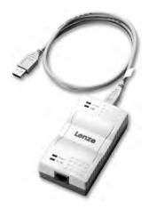
USB diagnostic adapter incl. connecting cable to the PC
