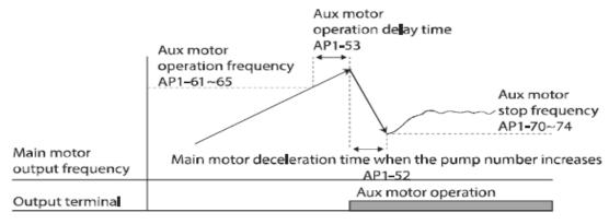
Auxiliary motor operation sequence by increased load
