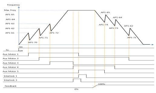
Interlock operation(Op time Order) when Operable Motor and Standby Motor are set to 3 and 2 each
