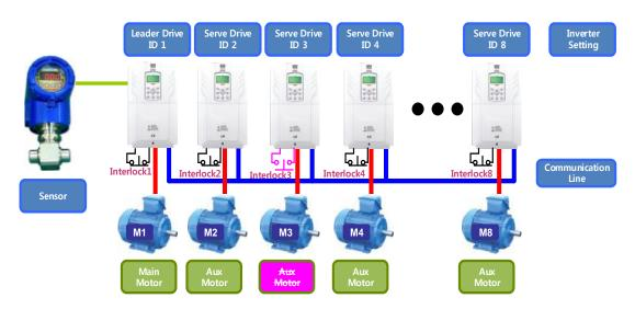
The picture below shows the function in case that M3 becomes HAND/OFF State or interlock and Trip are caused.(supposing that the priority is not changed),(interlock is the function corresponding to B terminal(Normal close)).
