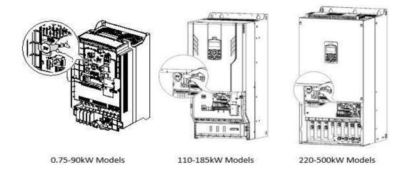
6 Reattach the front cover, the power cover, and the keypad back onto the inverter body
