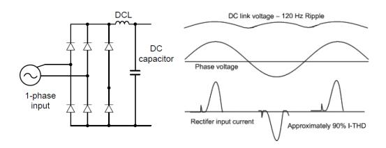
Figure-2 Typical Single-Phase Configuration
