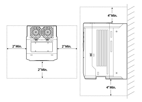
• Ensure sufficient air circulation is provided around the inverter when it is installed. If the inverter is to be installed inside a panel, enclosure, or cabinet rack, carefully consider the position of the inverter's cooling fan and the ventilation louver. The cooling fan must be positioned to efficiently transfer the heat generated by the operation of the inverter.
