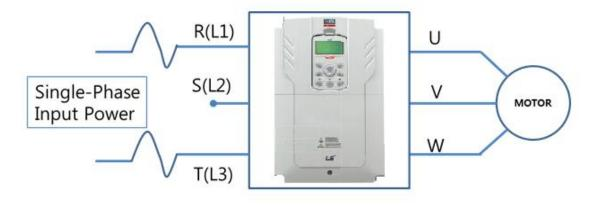
Figure-3 Terminal Wiring Diagram
