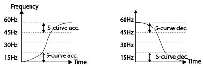
[Acceleration / deceleration S-curve pattern configuration]
