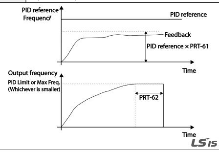
In the graph above, Pipe Break occurs if the feedback is smaller than the value calculated by multiplying the two values set at PID-04 and PRT-61(PID-04 x PRT-61) at the inverter's maximum output (when PID output is the maximum set value, or the inverter is running at the frequency set at DRV-20).
