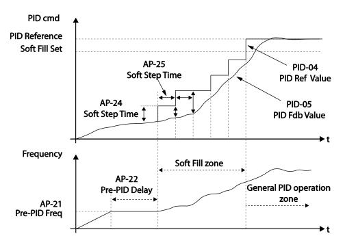
When a PID process is performed after the soft fill PID operation, the PID Reference value becomes the PID-11 PID Ref1 Set value.
