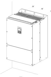
4 Install the two lower mounting bolts. Ensure that the inverter is placed flat on the mounting surface, and that the installation surface can securely support the weight of the inverter.
