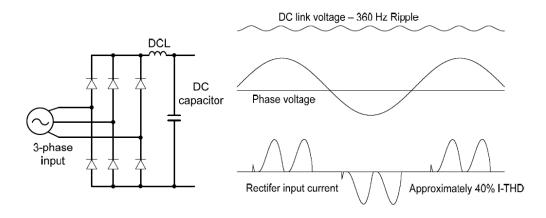
Figure-1 Typical Three-Phase Configuration
