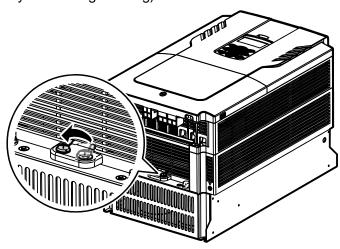
If the EMC filter is required in the future, reverse the steps and connect the EMC ground cable to the right terminal to enable the EMC filter.
