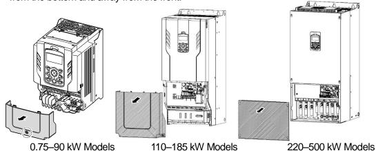
2 Push and hold the levers on both sides of the cable guide (**①**) and then remove the cable guide by pulling it directly away from the front of the inverter (**②**). In some models (37~90kW) where the cable guide is secured by a bolt, remove the bolt first.
