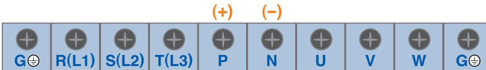
●● 22~30kW (30~40HP) <Built-in DC Reactor Type, 400V Class>
