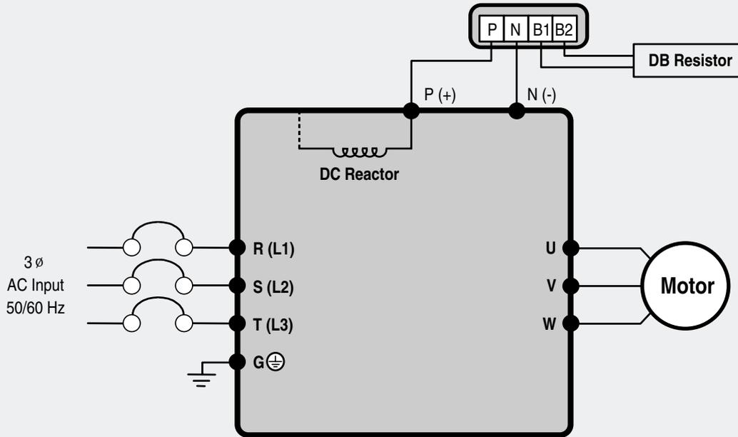
⚡ For 37~90kW (50~125HP) Built-in DCL Type
