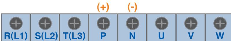
●● 37~90kW (50~125HP) / 110 ~280kW (150~350HP) <Built-in DC Reactor Type, 400V Class>
